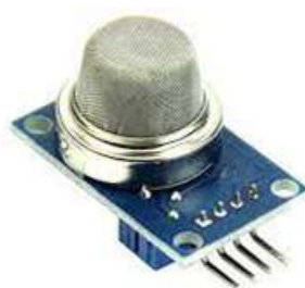
Fig .3: Gas Sensor.
